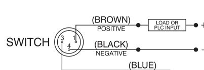
Typical Current Sinking (NPN) Configuration
