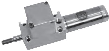
The Bimba Original Line Rod Lock Cylinder is a normally clamped unit that holds the piston rod in position when air pressure is not present. It is ideal for preventing drift at machine shut down.
