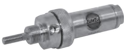
The all stainless repairable Original Line cylinders are ideal for food processing, chemical, medical, pharmaceutical, offshore or marine equipment, and energy production or waste management applications. The bell ring design also offers the added benefit of full reparability without the need for hand tools by securing the body to the rod guide with a knurled, threaded nut.
