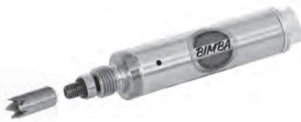
Our rugged hole punch cylinder has been redesigned with a removable cutter to allow customers to replace the cutter as needed without having to replace the entire cylinder. The razor sharp cutting teeth are designed to punch millions of holes in thin plastic film.
