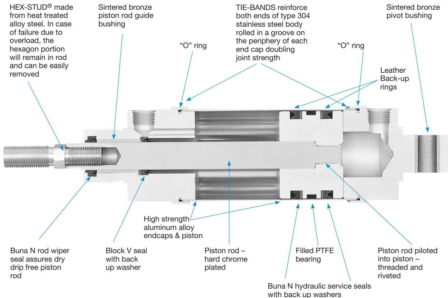
The Bimba "500" is a precision built, compact, lightweight hydraulic cylinder designed specifically for hydraulic use only, at pressures up to 500 psi.
